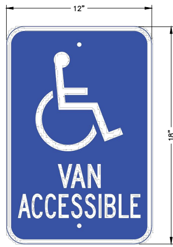
ACCESSIBLE SIGNAGE DETAIL
